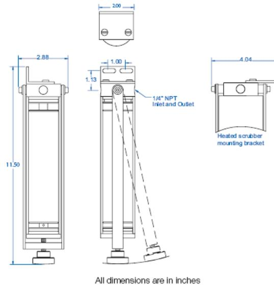
Mount scrubber in a vertical orientation using the angle bracket provided. Connect gas sample lines to the labeled inlet and outlet ports. Be sure to connect sample inlet to port marked "IN" on the scrubber housing
