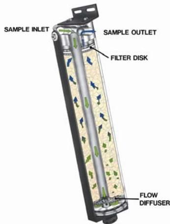
Phosphoric acid is very hygroscopic so it will draw water from the gas stream, creating some liquid phosphoric acid solution in the bottom of the scrubber. To avoid excess liquid formation, the scrubber should be heated, either by installation in a heated enclosure or by using a heated scrubber.
