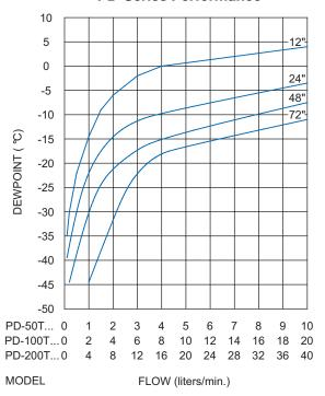
Conditions: Inlet dew point of 20°C, purge flow rate 2 times sample flow
